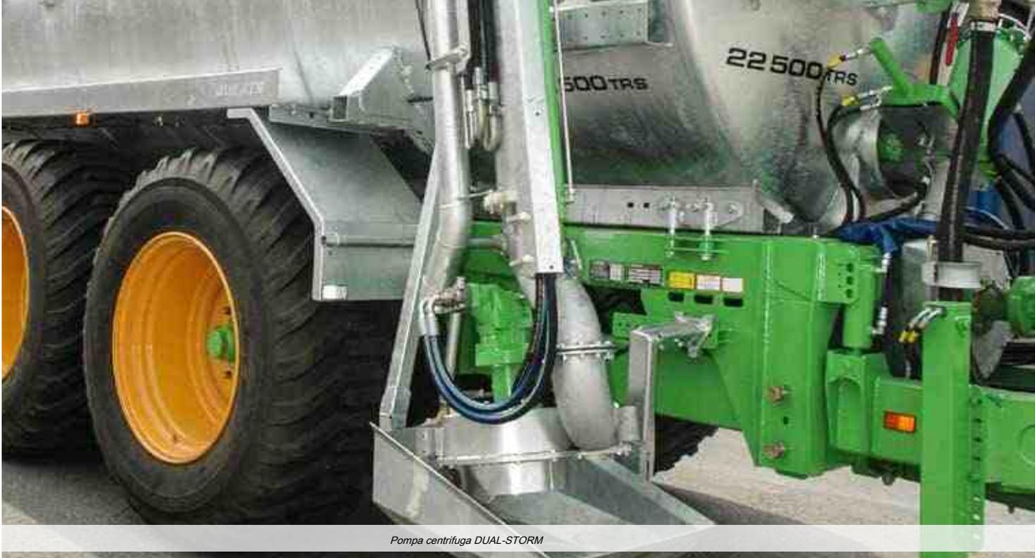
Pompa centrifuga DUAL-STORM
