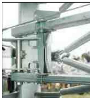
Once the injector is folded, the elements that are located on the upper arms are maintained in position by a locking system. A simple notch prevents each element from making a rotation round its axis and from falling down. The elements remain thus very rigid in relation to the vibrations due to transport.
